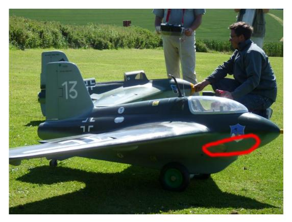
On the photo above you see one of the two screened inlets to the left of the red circle. In our opinion the location is to far aft and should be more in front in order to increase the ram-air effect. This would, on the other hand, be a valid location for a Naca scoop. Try NOT to open the side windows even if the plans say so. Should you have any questions please call us at 919-533-6275 in order to discuss this subject and in order to get the latest information.
